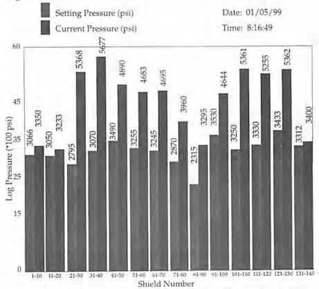
Figure 2. Setting and current average pressure distribution for every ten shields.
