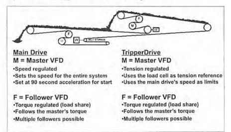
Figure 3. Main and tripper drive control systems.
