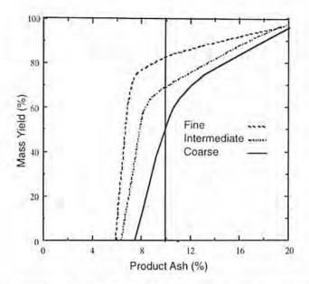
Figure 1. Typical yield-grade curves for a three-circuit coal preparation plant using conventional cleaning circuits producing equal grade products from the individual circuits.
