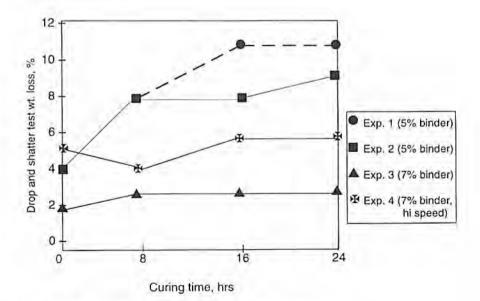
Figure 5. Effects of curing time on the strength of briquettes.
