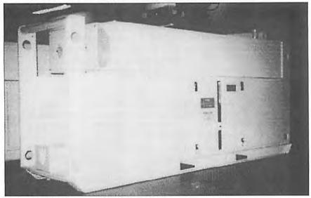
Figure 1. VFD drive controller.
