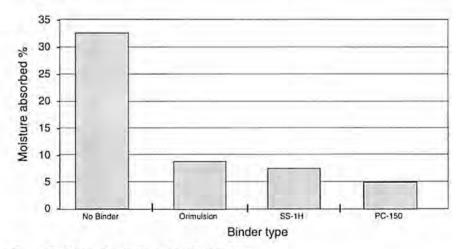
Figure 3. Water absorption of coal briquettes.
