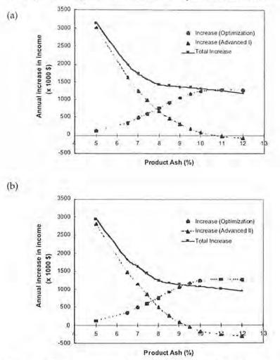
Figure 5. Predicted (a) annual income and (b) increase in annual income for the optimized plant with the existing cleaning circuits and the advanced cleaning circuits for the treatment of coal from the Herrin (Illinois No. 6) seam.
