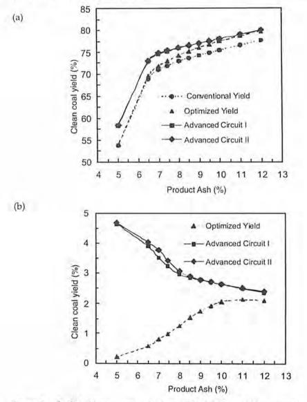
Figure 4. Predicted improvements in clean coal (a) yield and (b) incremental yield on the basis of product ash content for the optimized plant with the existing cleaning circuits and the advanced cleaning circuits for the treatment of coal from the Herrin (Illinois No. 6) seam.
