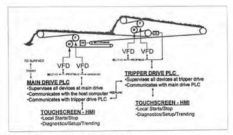
Figure 4. Equipment layout of control system.
