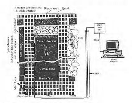
Figure 1. Schematics of surface data acquisition system.
