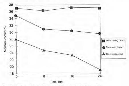
Figure 4. Effects of curing time on moisture content of briquettes.
