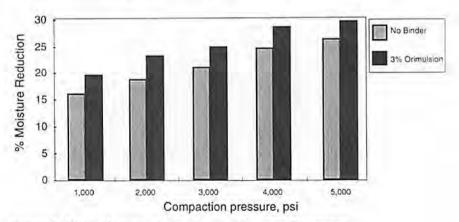
Figure 2. Effect of compaction pressure on fine coal dewatering.
