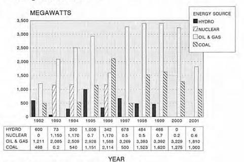
Figure 4. Planned utility additions by energy source.
