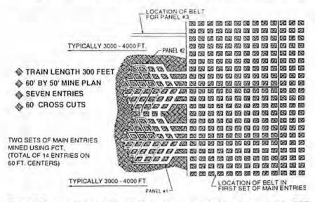
Figure 7. Commercial mine plan and belt takeup to maximize utilization of the FCT.
