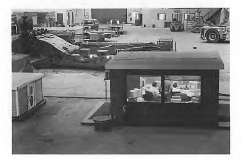
Figure 3. Experimental computer-assisted continuous mining machine, surface control center and underground control center. The machine and underground control center supported underground experiments from January, 1991 to January, 1993.
