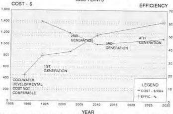
Figure 10. Clean coal technology demonstration program, projected cost and efficiency of commercial units.
