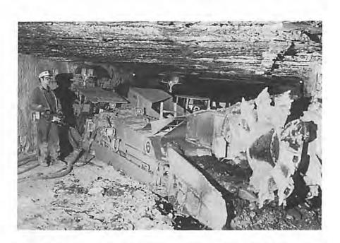
Figure 2. An operator controls a continuous mining machine using a radio remote control, "pendant" console-levers and switches hanging from a neck strap. Being able to relocate the operator to a haven of safety is the Bureau's research goal.
