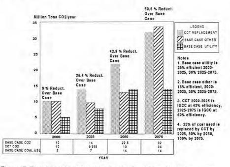
Figure 13. Potential world wide carbon dioxide reductions - efficiency improvements.
