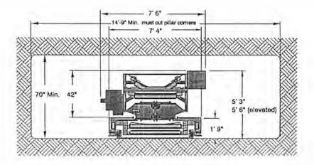
Figure 4. Cross-section of the 3FCT on the conveyor belt.
