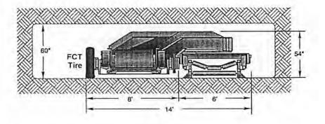
Figure 6. 3FCT and low frame, side by side discharge.
