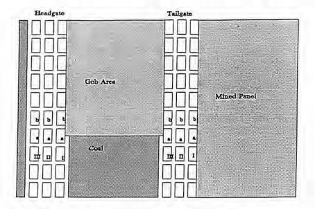
Figure 7. Illustration of longwall with four-entry development.
