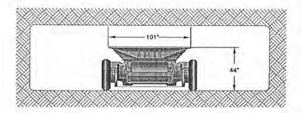
Figure 5. The 3FCT inby unit hopper.
