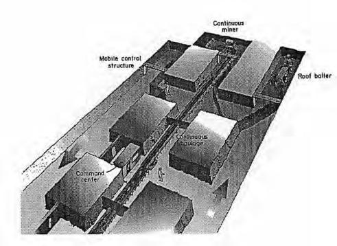
Figure 1. Conceptualization of targeted room-and-pillar mining scenario.
