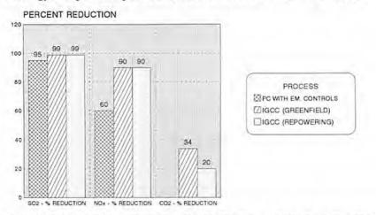
Figure 8. Clean coal technology demonstration program, projected performance of capacity for IGCC power plants in greenfield applications and repowering applications.
