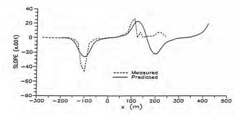
Figure 4. Tilt in x-direction along the monitoring line.
