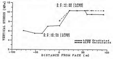
Figure 6. Average vertical stress over chain pillar on headgate using LGMM and ALPS techniques.
