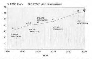
Figure 11. Projected performance of coal-based, combined cycle power systems.
