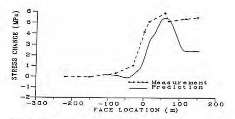
Figure 5. Stress change in the pillar adjacent to the face.
