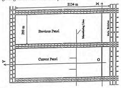
Figure 1. Mining layout for study panel.
