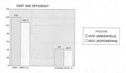
Figure 9. Cost and efficiency, projected performance of IGCC power plants compared to pulverized coal-fired power plants.
