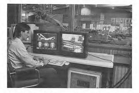
Figure 1. Computers and displays such as shown here will permit underground machine operators to control their machines while remaining safely away from danger.
