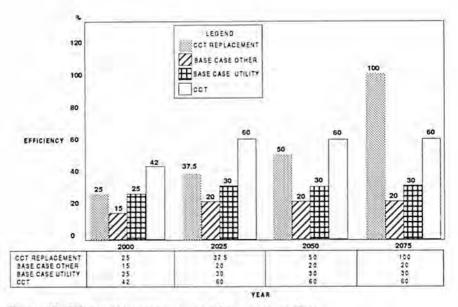
Figure 12. Efficiency improvements with new power plants.
