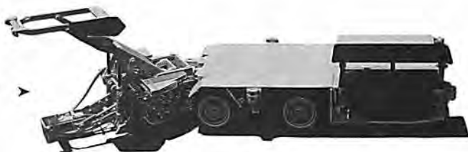
S-R Single- And Dual-Drillhead Roof Bolters In Rigid Or Articulated Frame Models
