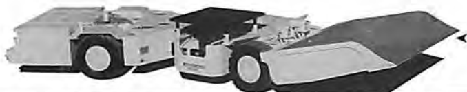
Battery-Powered Un-A-Tracs® With The Exclusive S-R X-90 Control System And Optional Radio Remote Control
