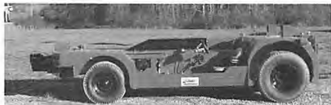
The GATOR II MPV drive train consists of a 58 H.P. MSHA certified engine, a 2 or 3 speed power shift transmission and a planetary rear axle.
