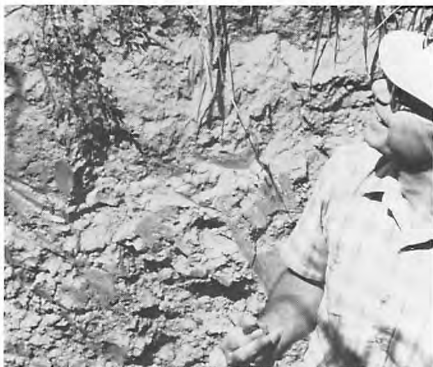
Fig. 2 — Availability of water should be a major criterion in building post-mining soils. Roots cannot grow into compacted mined or unmined subsoils to obtain water even if moist. Recognition of compaction problems may lead to new understanding of reclamation needs.
