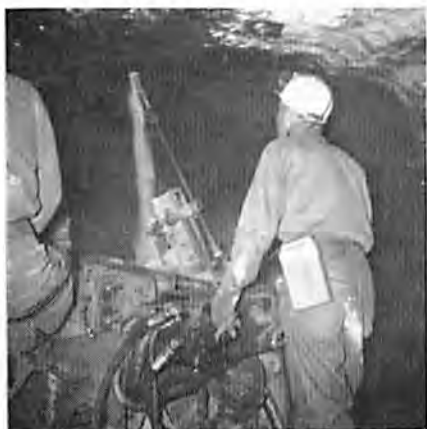
A roof bolter drills an angular hole to install a bolt on a 20-25° angle (note the 2½ ft. extension added to the drill stem). Bolts currently in use are ⅝ in. by 5 ft. long
