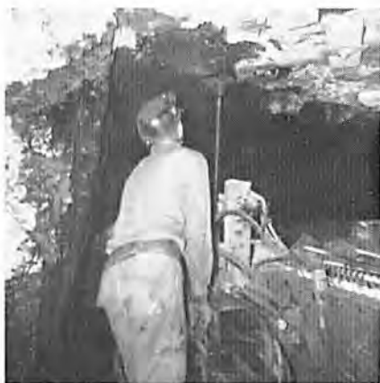
With a tightening wrench placed on the drill, the roof bolt is tightened under slow feed. The relief valve at slow feed cuts off at 1000 psi which develops a torque on the bolts from 150 to 160 ft. lb.
