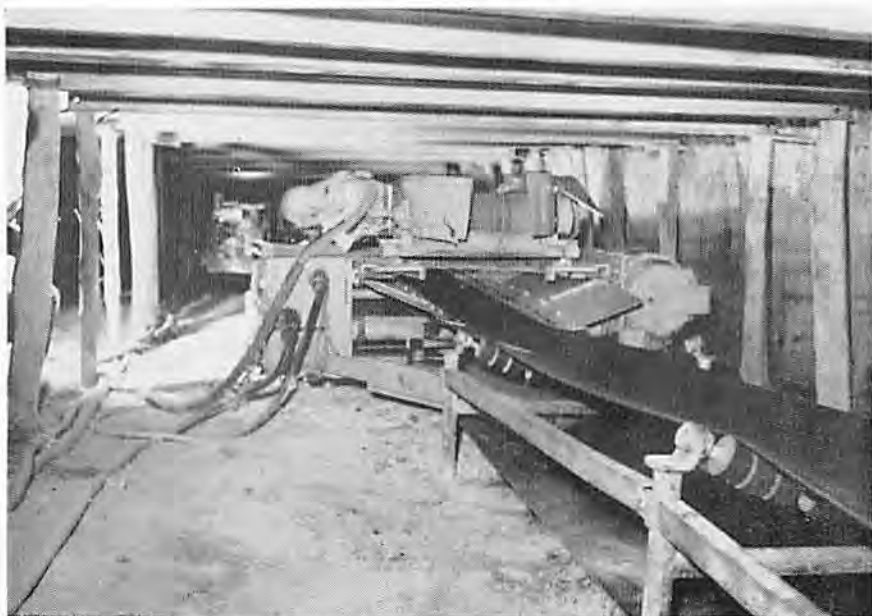
The extensible belt in operation provides an intermediate haulage system as near to continuous haulage as is possible with present day mechanical equipment
