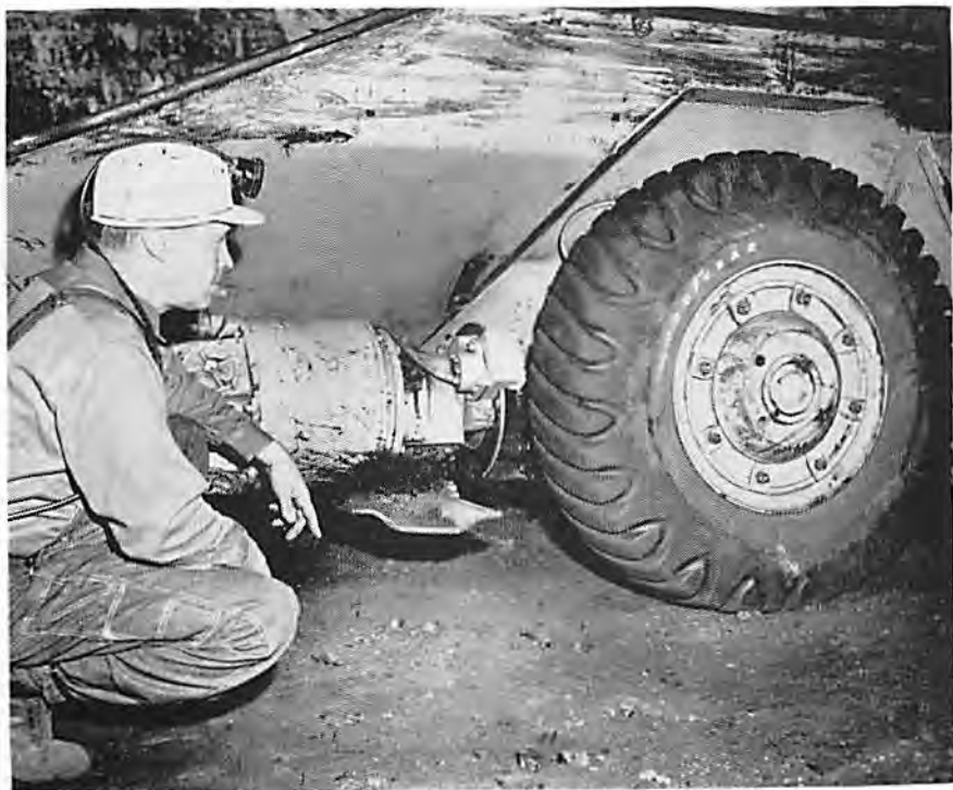
Shuttle-car tires should be inspected daily. See that they have sufficient air pressure and look for damage. Change those found to be bad.
