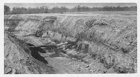
Fig. 5. The results of inadequate stemming
