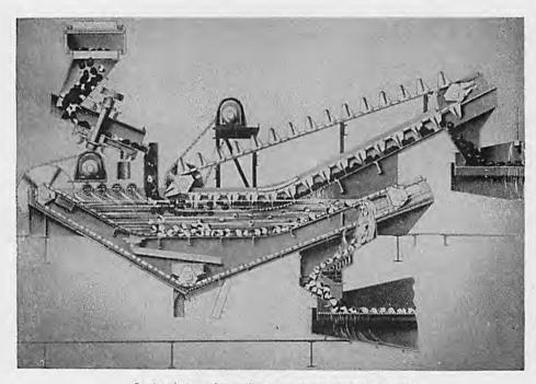
Sectional view of McNally-Tromp heavy density bath unit
