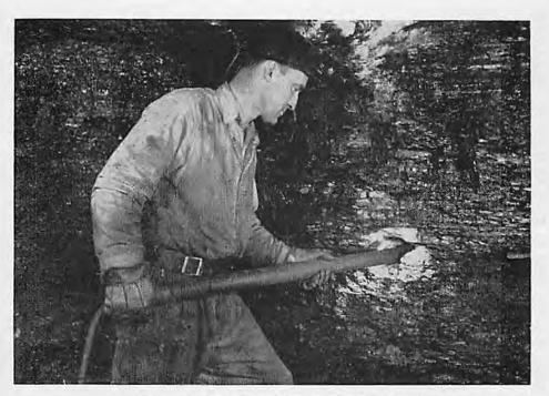
Fig. 4. Placing the assembled tube in the shot hole
