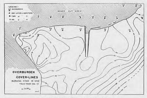
Fig. 1. Overburden contour at Burning Star Mine
