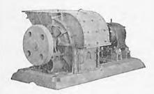
The "5" type crusher for reducing efficiently R. O. M. or lump to screenings in one operation. These crushers were designed to give constant and continuous operation.
