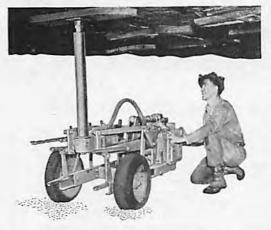
That's standard performance for electrically-operated CP MO-BILE ROOF BOLTING UNIT — RBD-30. This includes the complete bolting cycle — the hole is drilled and expansion bolt set without repositioning the unit — one motor drives both auger and bolt setter. Easy to operate under any condition — in high coal or seams as low as thirty inches.
