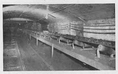
**RAY-MAN TENSION-MASTER** is the original conveyor belt made with rayon strength members designed for the super-tensions of long-lift mining. The ideal slope belt for eliminating transfer points to cut down coal breakage and increase belt life. Has extremely low stretch, half as much as conventional belts. Mildew and moisture proof.
