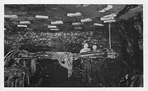
Fig. 1. Water applied to electric rotary drill eliminates dust
