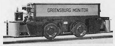
Double knee-action; better trackability. Floating power; less power consumption. Quick acting footbrake—essential for quick stopping, especially behind loading machines. Brake shoes that follow wheels (due to knee-action). Adjustable Timken Bearings throughout.
