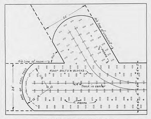
Fig. 2. Sketch showing roof bolt pattern in rooms
