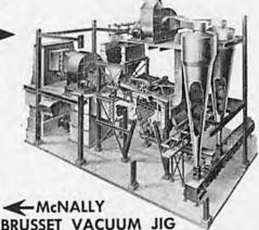
The Brusset Fine Coal Dry Cleaner, a completely self-contained unit, is noted for greater capacity per
