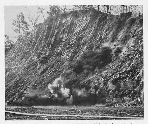
Fig. 6. A single shot detonated at the back of a horizontal hole with adequate stemming
