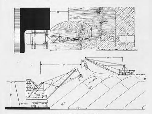
Fig. 3. Enos digging and spoil plan
