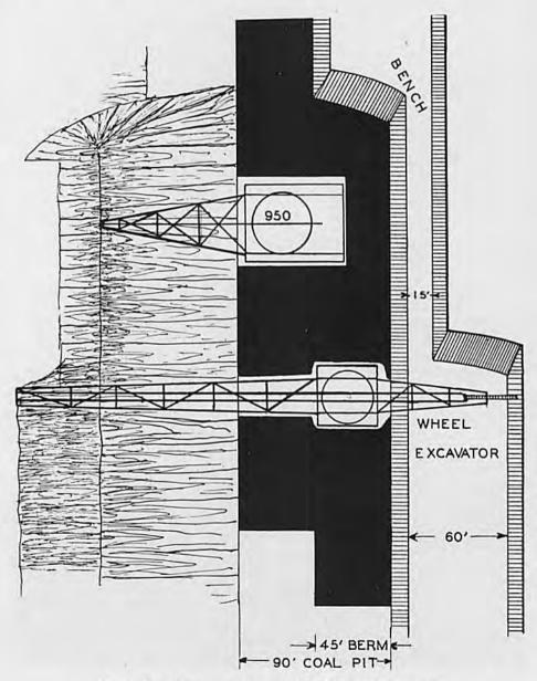
Fig. 2. Plan of working tandem units-United Electric Buckheart Mine
