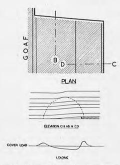
Diagram showing area and width of maximum pressure arch
