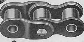
COMBINATION OFFSET LINK—An Offset Link and a Roller Link assembled and riveted together, the pin being a press fit in the
