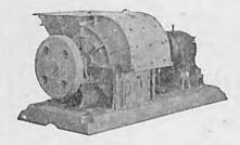
The "S" type crusher for reducing efficiently R.O.M. or lump to screenings in one operation. These crushers were designed to give constant and continuous operation.
