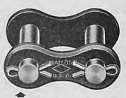
CONNECTING LINK—Cotter Pin Type—Standard for roller chains  $\frac{3}{4}$ " to  $\frac{2}{2}$ " pitch inclusive. The pins are riveted into one link plate; the "cover plate" is driven evenly into place over the drilled pin ends and is not a loose, or slip, fit. The cotters do not hold the link plate in place. The press-fit between pins and cover plate prevent the pins from turning and the plate from coming off.
