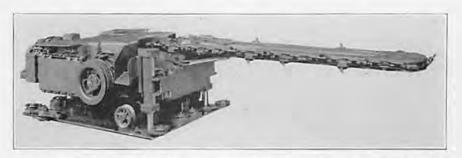
A modern Shortwall Top Cutter, mounted on hydraulic jacks for cutting above the floor of the mine.
