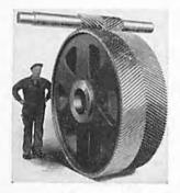
CONTINUOUS TOOTH HERRINGBONE GEARS and SPEED REDUCTION UNITS FOR ALL PURPOSES
