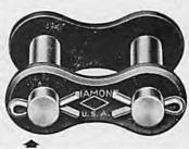
CONNECTING LINK—Cotter Pin Type—Standard for roller chains ¾" to 2½" pitch inclusive. The pins are riveted into one link plate; the "cover plate" is driven evenly into place over the drilled pin ends and is not a loose, or slip, fit. The cotters do not hold the link plate in place. The press-fit between pins and cover plate prevent the pins from turning and the plate from coming off.
