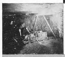
shattercracks...increases realization...reduces cleaning costs. Protection against overshooting is positive. Roof troubles are reduced. Because crews can enter the working face immediately after the fall, non-productive time of men and machines is greatly reduced.
