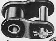
OFFSET LINK—(Half Link)—Used (one per chain) when the chain length requires an odd number of pitches. The use of offset links should be avoided whenever possible and if their use is necessary the "combination" offset link is to be preferred particularly for the short pitch chains and chains run at high speeds or under heavy loads.
