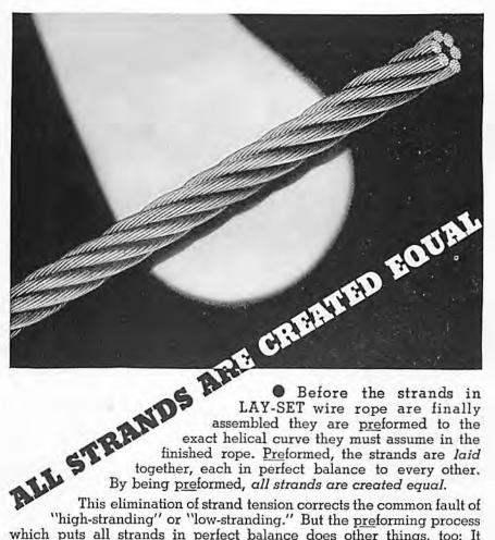
Before the strands in LAY-SET wire rope are finally assembled they are preformed to the exact helical curve they must assume in the finished rope. Preformed, the strands are laid together, each in perfect balance to every other.
