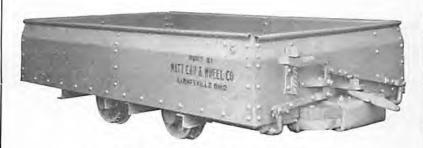
Here is a modern all steel car carrying a pay load of 6.000 lbs. which replaced old wooden cars having a capacity of only 3,000 lbs.
