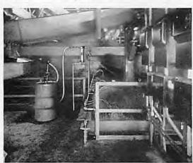
Ideal Lubrication applied to Shaking Screen Drives modern Pennsylvania coal preparation plant of large Bituminous Producer.
