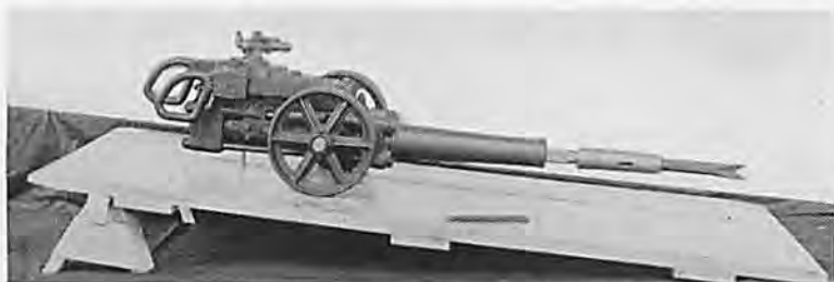
A puncher of the type described by the author. The drift pin on the board was used for loosening the pick.
