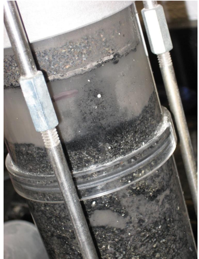
Water worm holing can be an issue giving erroneous results
