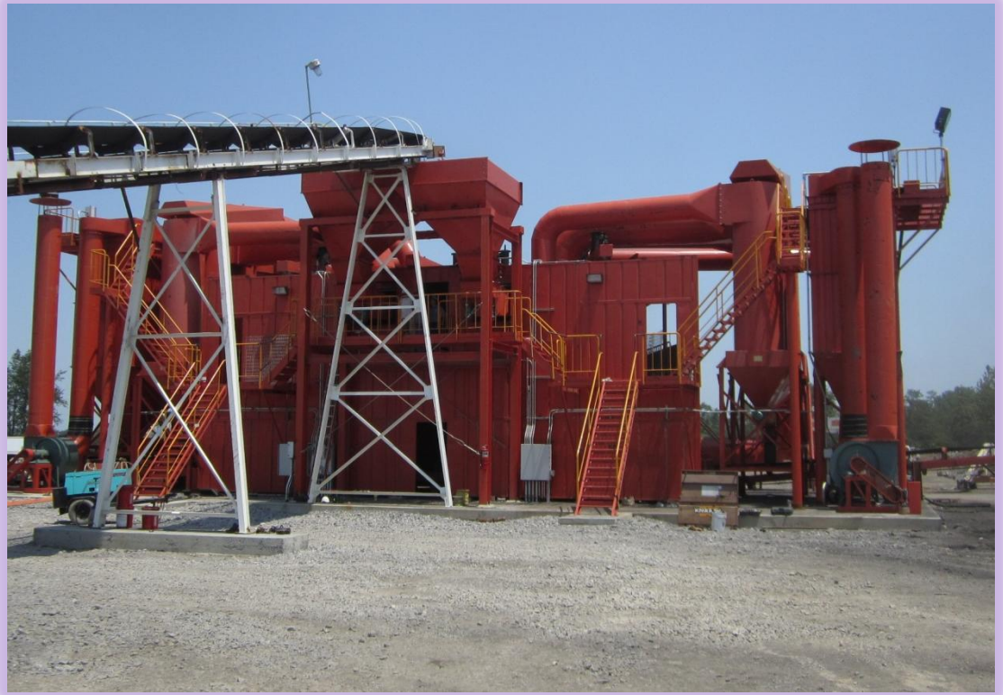
Illinois FGX Separator Installation 250 TPH capacity
