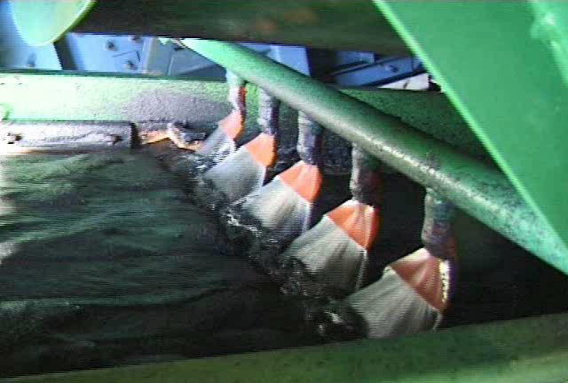
Action of Stack Sizer Repulp Trough
