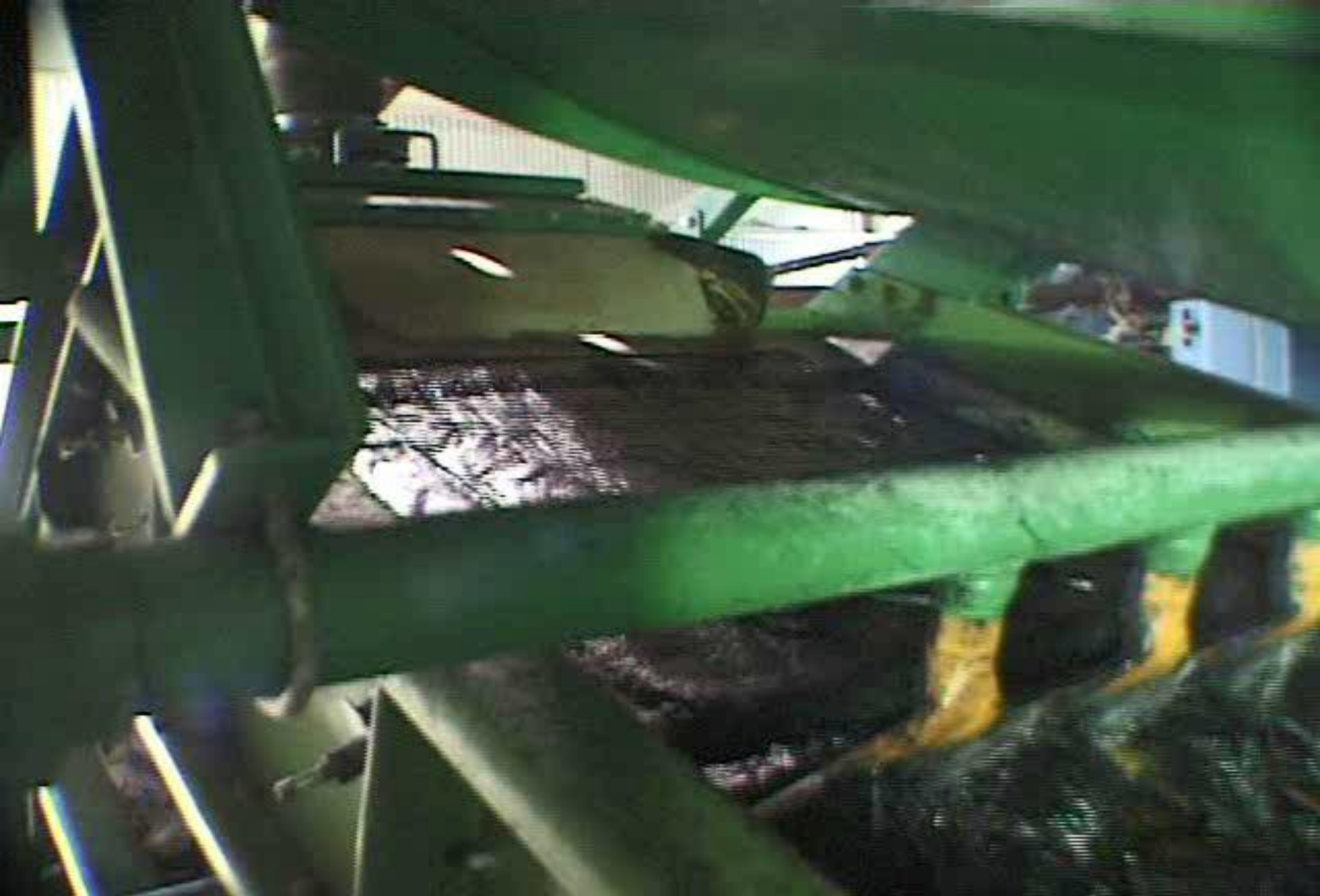
Coal Sizing on 100 micron Urethane Panels
